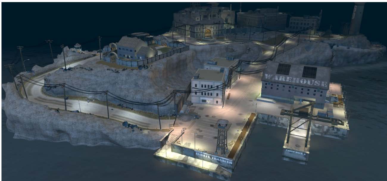
Figure 1: Inferred lighting allows this complex scene with 213 active lights to be rendered at 1280x720 resolution, with 8x MSAA, at 23fps (43.5ms) on a GeForce 8800GTX.
