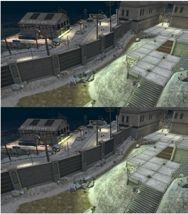
Figure 9: A scene with 122 dynamic lights. Using an 800x450 L-buffer with a 1280x720 8x MSAA framebuffer and DSF (Top) results in both better quality anti-aliasing and faster framerate (40fps vs 31fps) than using a 1280x720 L-buffer with no DSF (Bottom).
